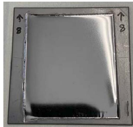
Figure 9 - Electropolished 2" x 2" tantalum coupon. Edge shows surface prior to polishing.
