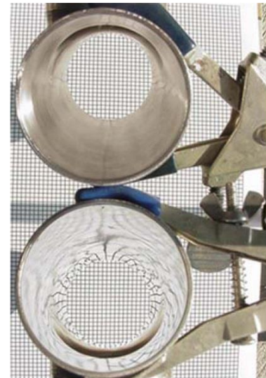
Figure 7 - 316SS tube surface before (top) and after (bottom) sequenced pulse reverse electropolishing in a \text{NaCl}-\text{NaNO}_3 electrolyte.
