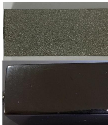
Figure 10 - Electropolished powder bed additively manufactured Ti-6Al-4V.
